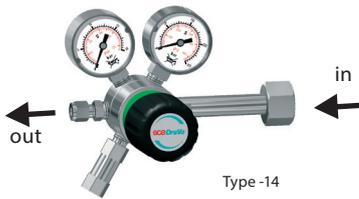
**Single-stage, for inert, reactive, flammable and oxidizing gases and gas mixtures, purity max. 6.0, cylinder pressure 315 bar/ 4500 psi, downstream pressure range 0.5 - 200 bar / 7 - 2900 psi**
