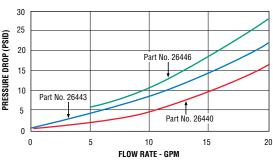
**FLOW HAIE - GPW**Tests conducted with units in vertical position (lead wires up) with water at +70°F (21°C).
