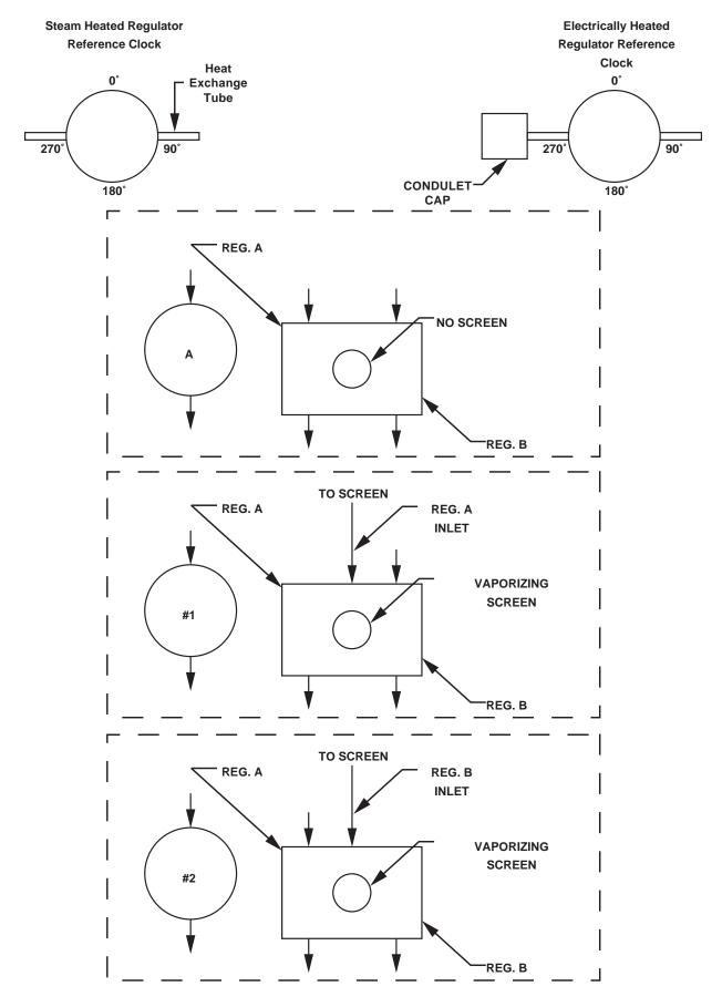
Location of ports from to of regulator "A". Arrow pointing toward body is inlet. Arrow pointing away from body is outlet.
