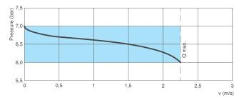
The plots are showing the reduced pressure falloff that occurs through the valve when the flow increases. Ensure that the operating conditions fall on the area depicted in blue for the recommended fluid flow velocity through the valve.
