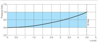
The plot is showing the increase in the upstream pressure that occurs through the valve, when the flow increases. Ensure that the operating conditions fall on the area depicted in blue for the recommended fluid flow velocity through the valve.
