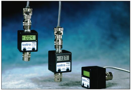
etra's Model LD 330 is a small Local Display designed to be easily installed in-line between a Setra pressure transducer and the user's data acquisition system and power supply. It has a low power consumption 3-1/2 digit analog to digital converter with a Liquid Crystal Display (LCD). The compact housing allows transducer and power supply connection through a variety of electrical terminations. The LD 330 is factory calibrated
