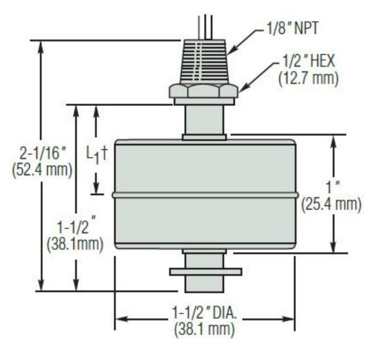
$L_1 = 5/8" (15.7 \text{ mm}) \text{ N.O.}; 3/4" (19.1 \text{ mm}) \text{ N.C.}$
