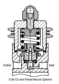
Panel mount option requires 1.39 (35.3mm) minimum diameter panel cut out
