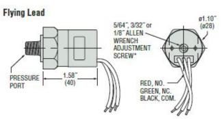
\* Adjustment screw is located under protective screw.
